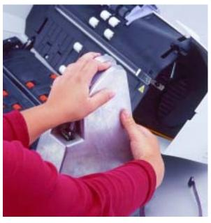
18. Thread the imprinter cable through the opening and into the imprinter area.
